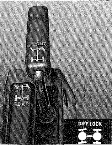
▲ Optional front and rear diff locks maintain traction in difficult off-road conditions.
